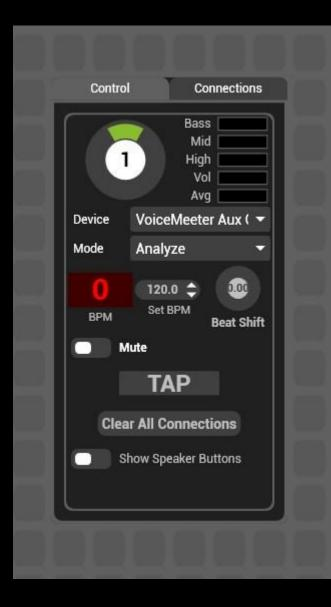
The BeatBridge component triggers parameters of Hippotizer in time with an audio source.
